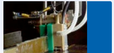
Phased Array Stringer Bubbler
