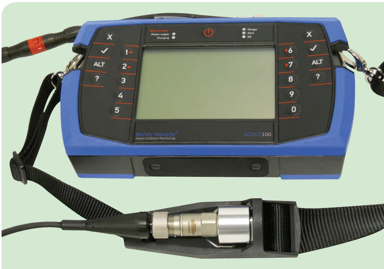
FIGURE 2: SCOUT's sensor keeper is a convenient place to carry the accelerometer, keeping it clean and providing a ferrous "keeper" for the magnetic circuit of the mounting base.
