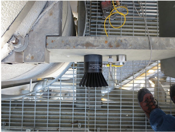
FIGURE 1: Warm Gland Seal Condenser support structure, with magnetically-mounted Power Puck and the thermocouple being used to monitor surface temperature for data collection. The temperature signal was processed and transmitted by the wSIM that the Power Puck was energizing.
