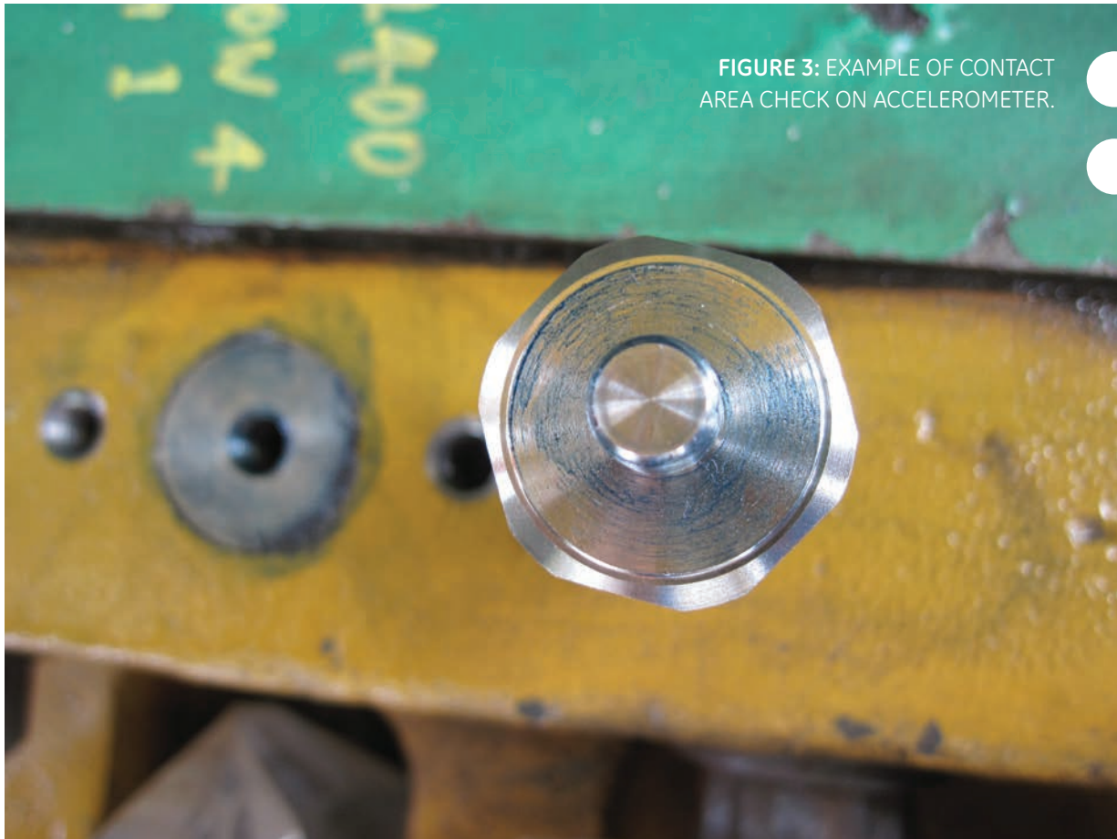
FIGURE 2: Accelerometer and Housing Mounting Details
