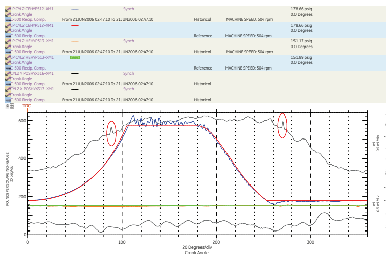
FIGURE 7: The vertical piston rod vibration signal (top grey line) shows two spikes that are symmetrical with respect to BDC.
