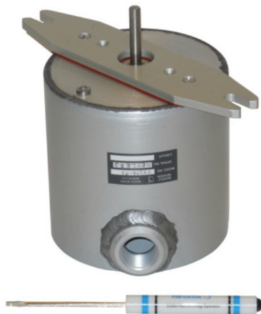
FIGURE 9: Rotary Potentiometer, with a small 135 mm (5.3 in) long screwdriver for size reference. The shaft that is visible extending from the top of the potentiometer housing is attached at the end of the camshaft, and rotates as the camshaft rotates.
