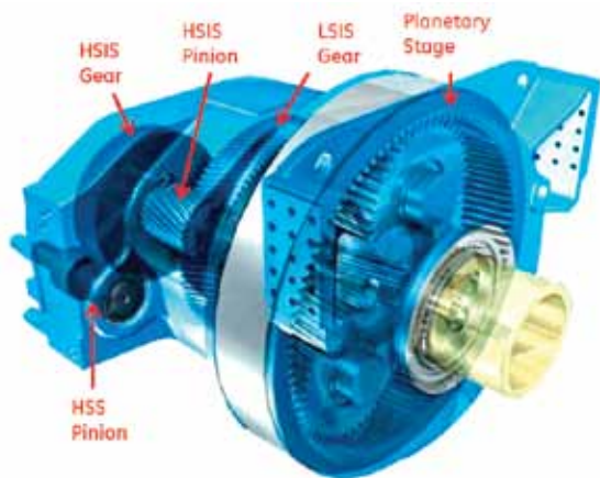
FIGURE 4: Wind turbine planetary gearbox design
