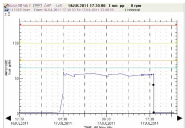
FIGURE 7: Normal vibration amplitudes observed at the DE Y probe after remedial work.
