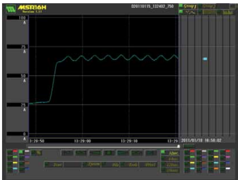
FIGURE 3: Motor Current Trend Plot of the B Motor. Observe that the frequency of the current fluctuation is approximately 0.35 Hz (3.5 cycles/10 seconds).
