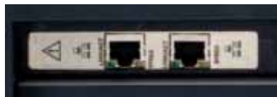
FIGURE 1: ADRE 408 communication ports.
