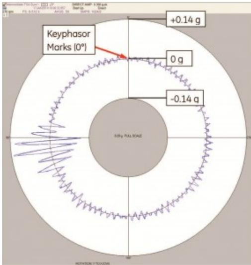
FIGURE 2: In this example, the same data from Figure 1 is shown in a wrapped timebase plot. The accelerometer is mounted vertically on the top of the monitored gearbox, where the 0 degree reference mark is shown on the plot. Rotation is clockwise, so, starting with the Keyphasor event, time increases (degrees of shaft rotation increase) in the counterclockwise direction around the outer circle of the plot. With machine speed of 276 rpm, each complete revolution takes about 0.217 seconds.
